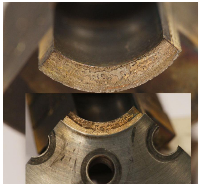
Fig. 15. Highlight of joint failed on the right side of Fig. 14.
