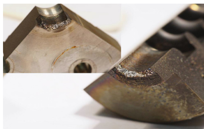
Fig. 16. Highlight of molybdenum “extension tubes” failed adjacent to the SST flange on the left side of Fig. 14.
