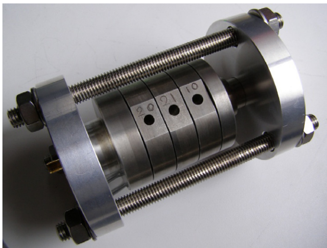
Fig. 7. Picture of the molybdenum structure under test.
